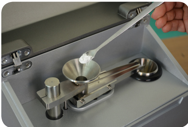
Dry dispersion and feeding system
